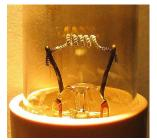
Fig. 2 Fluorescent light filament
